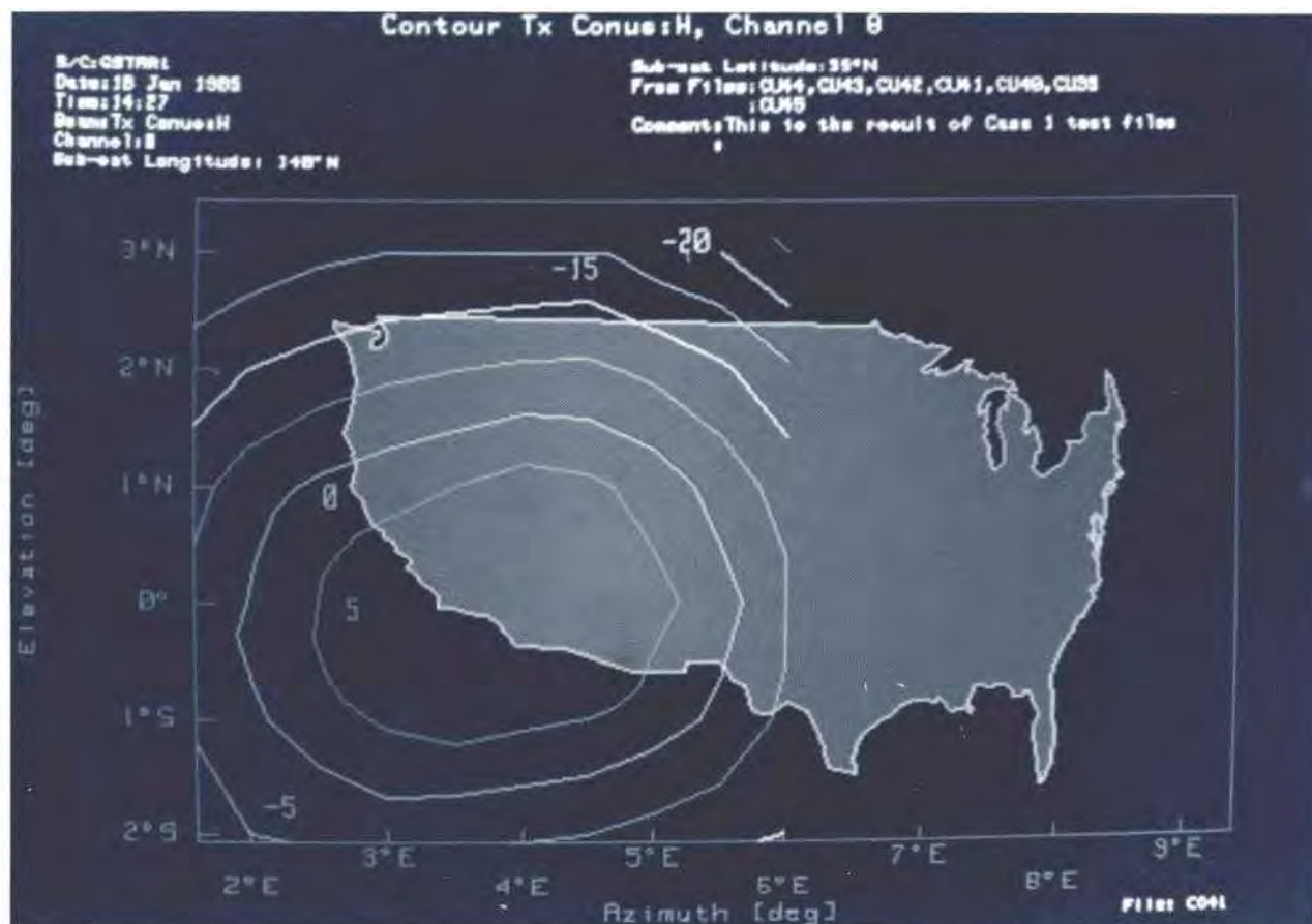
Figure 21. Antenna pattern and coverage area can be displayed in spacecraft or geometric coordinates
