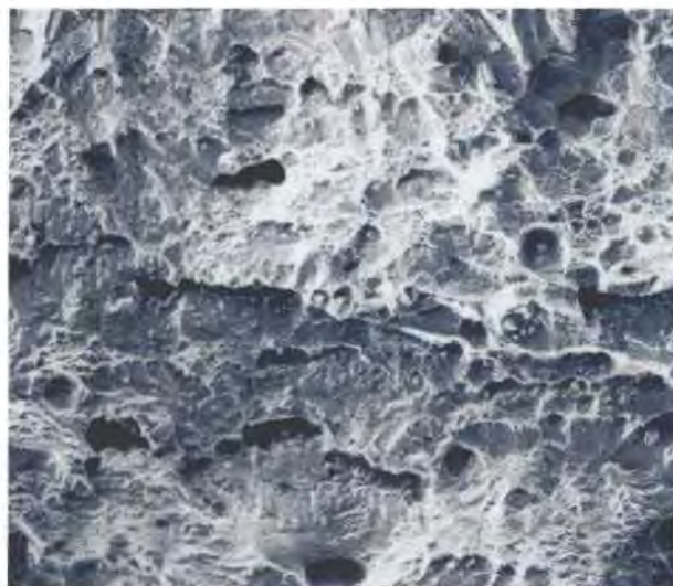
(a) Ductile (high-strength) failure resembles pulled taffy (350X)
