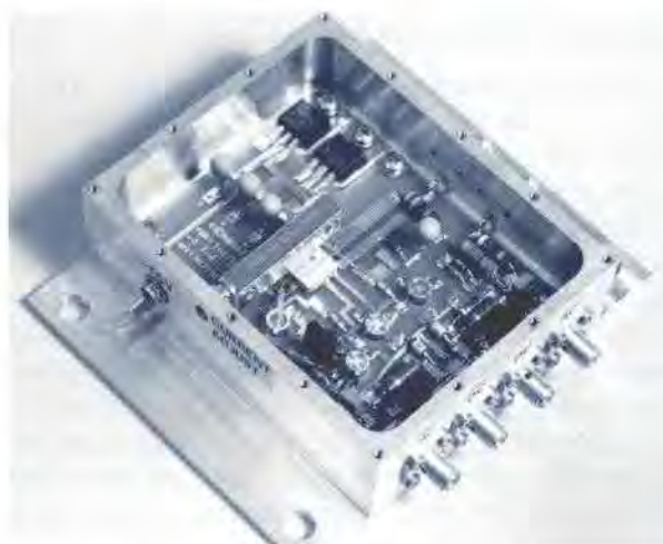
Figure 1. High-speed, high-current digital laser driver operates at 420 Mbit/s
