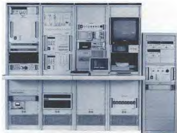
Figure 4. The TDMA System Monitor measures critical characteristics of TDMA bursts at radio frequencies
