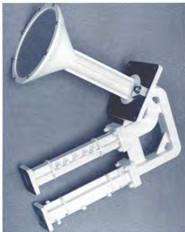
Figure 20. K_U -band feed system components are amenable to high-quantity/low-cost fabrication
