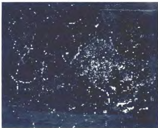
(b) Corresponding Auger electron map of chlorine
