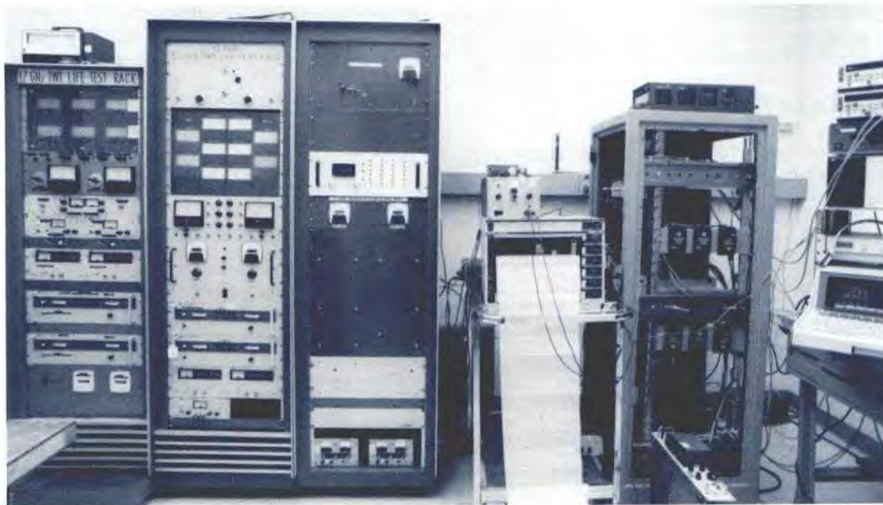
Figure 1. TWT life-test facility operates under computer control
