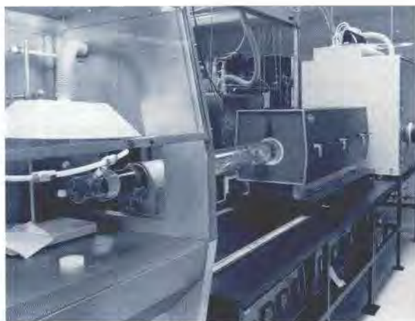
Figure 4. Computer-controlled halide epitaxial reactor for growing epitaxial layers on 50-mm-diameter GaAs wafers
