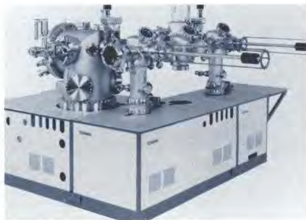
Figure 5. The Riber molecular beam epitaxy system will be used to develop the next generation of microwave and digital devices
