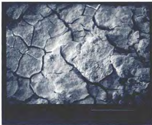
(a) Secondary electron image showing cracked mud appearance of green material
