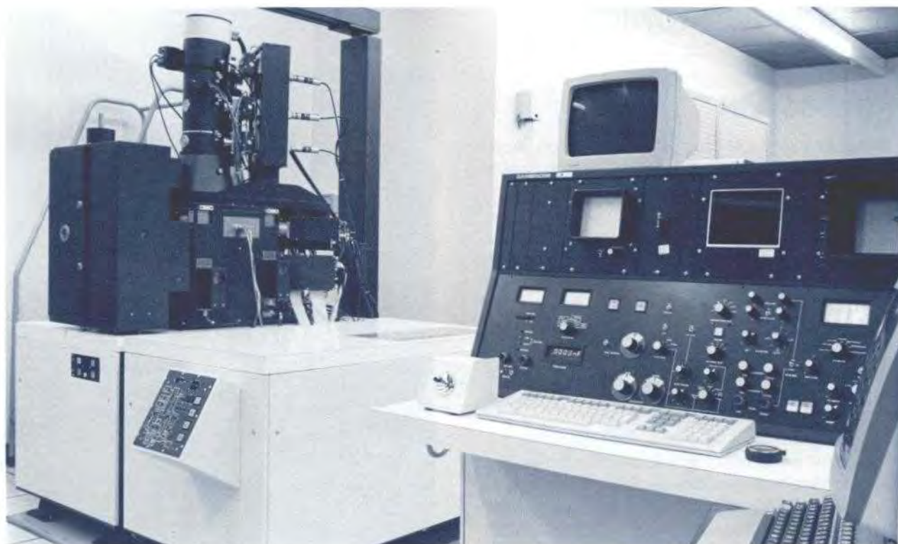
Figure 2. Operating console of the Cambridge Instruments, Inc., Electron Beam Pattern Generator
