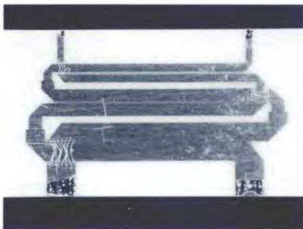
Figure 14. Novel 3-dB hybrid coupler results in a significant reduction in the size of balanced amplifiers
