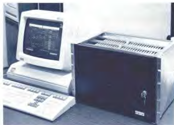
Figure 2. The Western Union Monitor and Control System allows an operator to monitor and control an entire TDMA network
