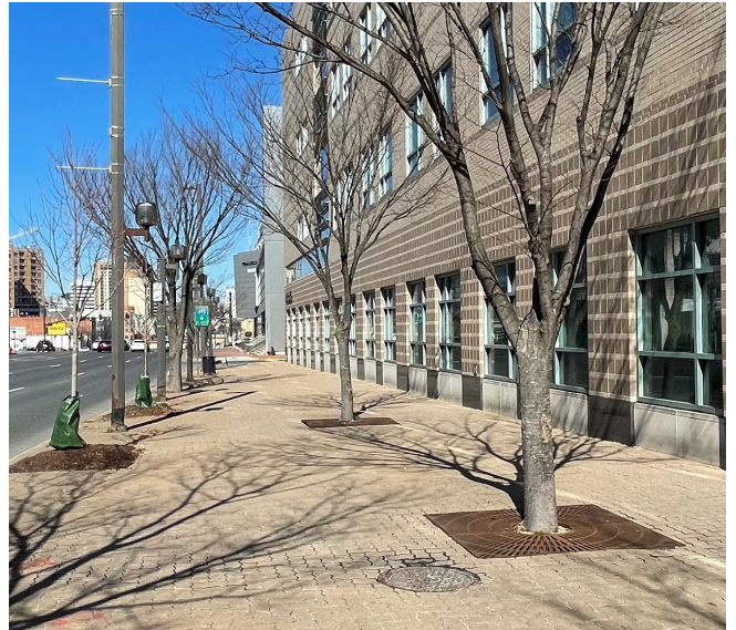
Georgia Avenue at Montgomery College: Street trees along the roadway have open planted areas while the trees in the wide sidewalk have planting areas covered with grates as pedestrians are likely to walk on them.
