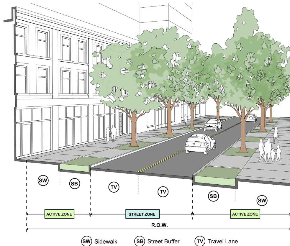
Illustrative section of a Downtown Street - Type B (constrained ROW)
