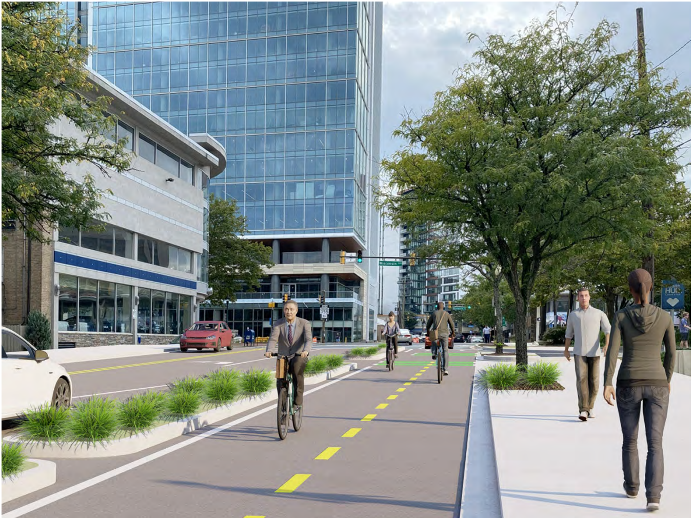
Figure 42: Rendering - Bikeway Facility Type Option 4 - Wide Two-way Separated Bike Lanes
