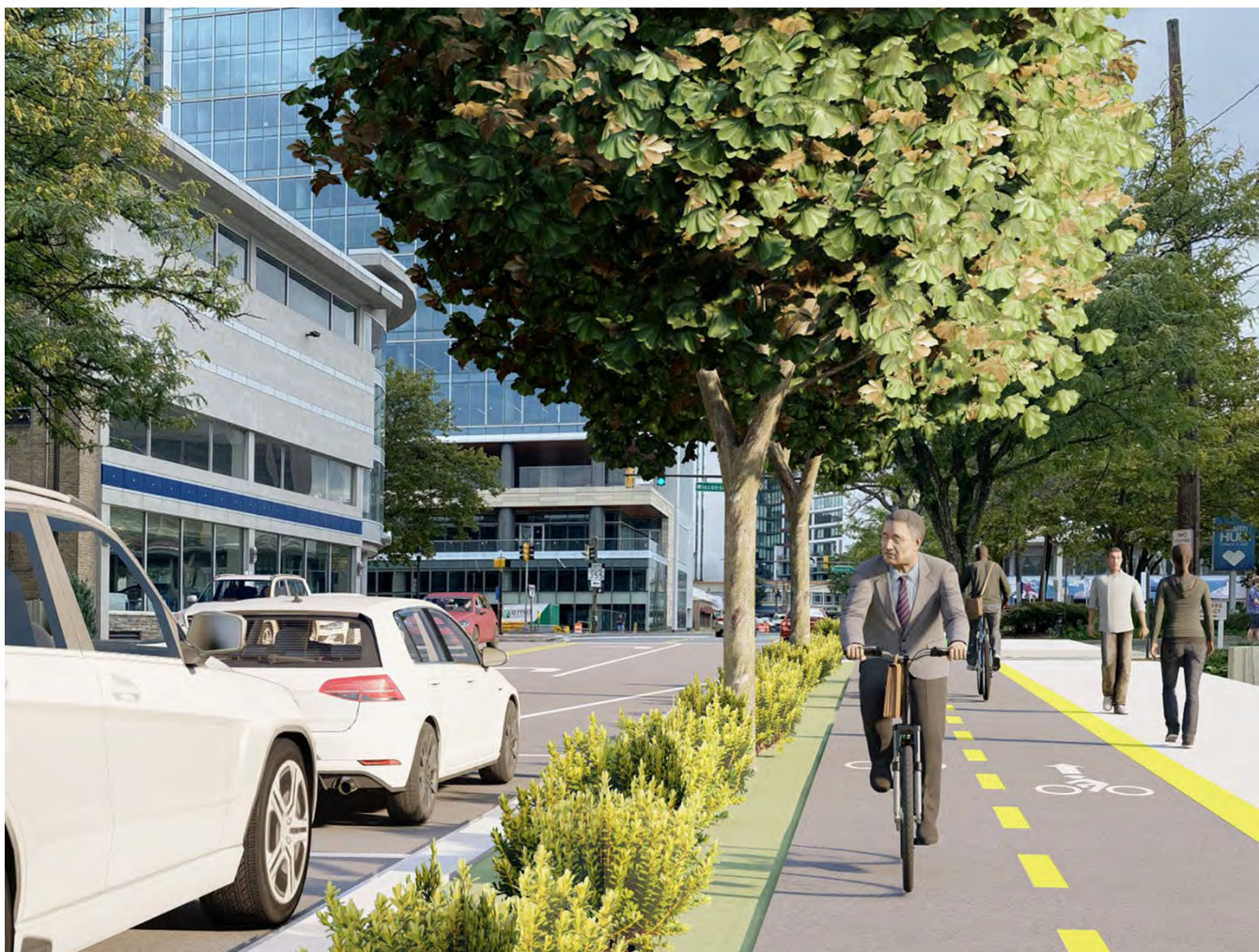
Figure 44: Rendering - Bikeway Facility Type Option 5 - Two-way Raised Separated Bike Lanes
