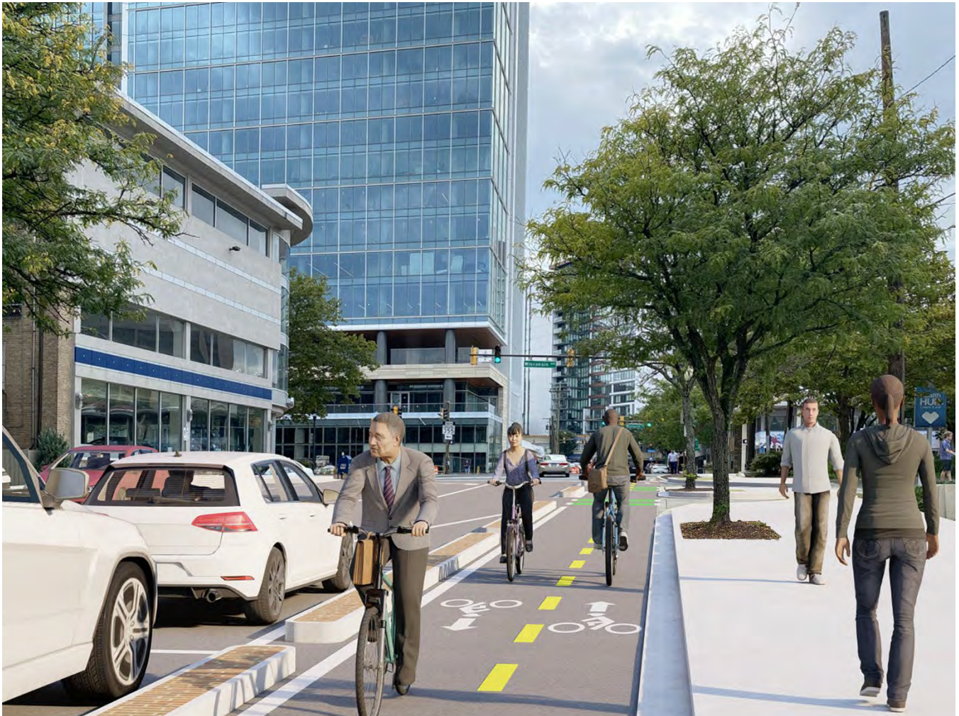
Figure 40: Rendering - Bikeway Facility Type Option 3 - Narrow Two-way Separated Bike Lanes
