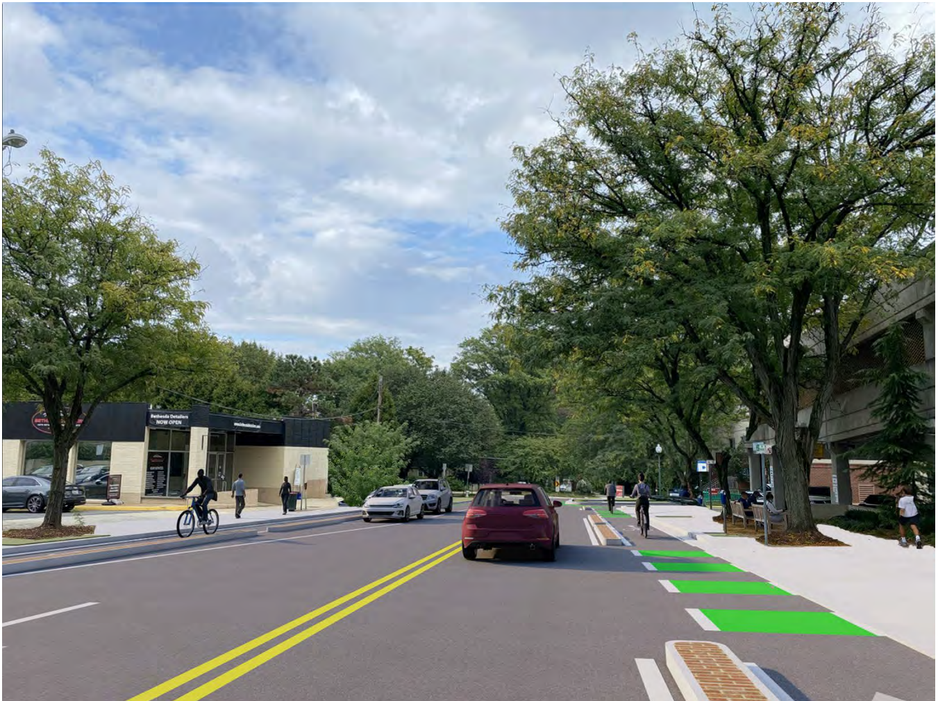
Figure 38: Rendering - Bikeway Facility Type Option 2 - One-way Separated Bike Lanes
