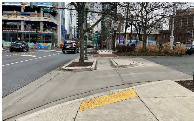
Sidewalks on Cheltenham Drive between Wisconsin Avenue and Tilbury Street are 10' wide with an additional 5' of tree-lined landscape buffer but are frequently interrupted by driveways.
