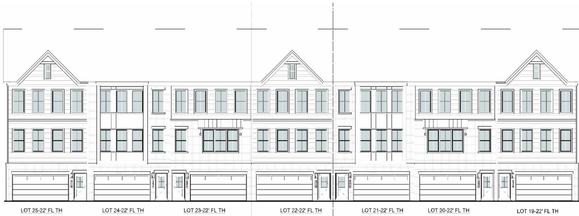
Figure 8: Typical Front-Loaded Townhouse Building String
