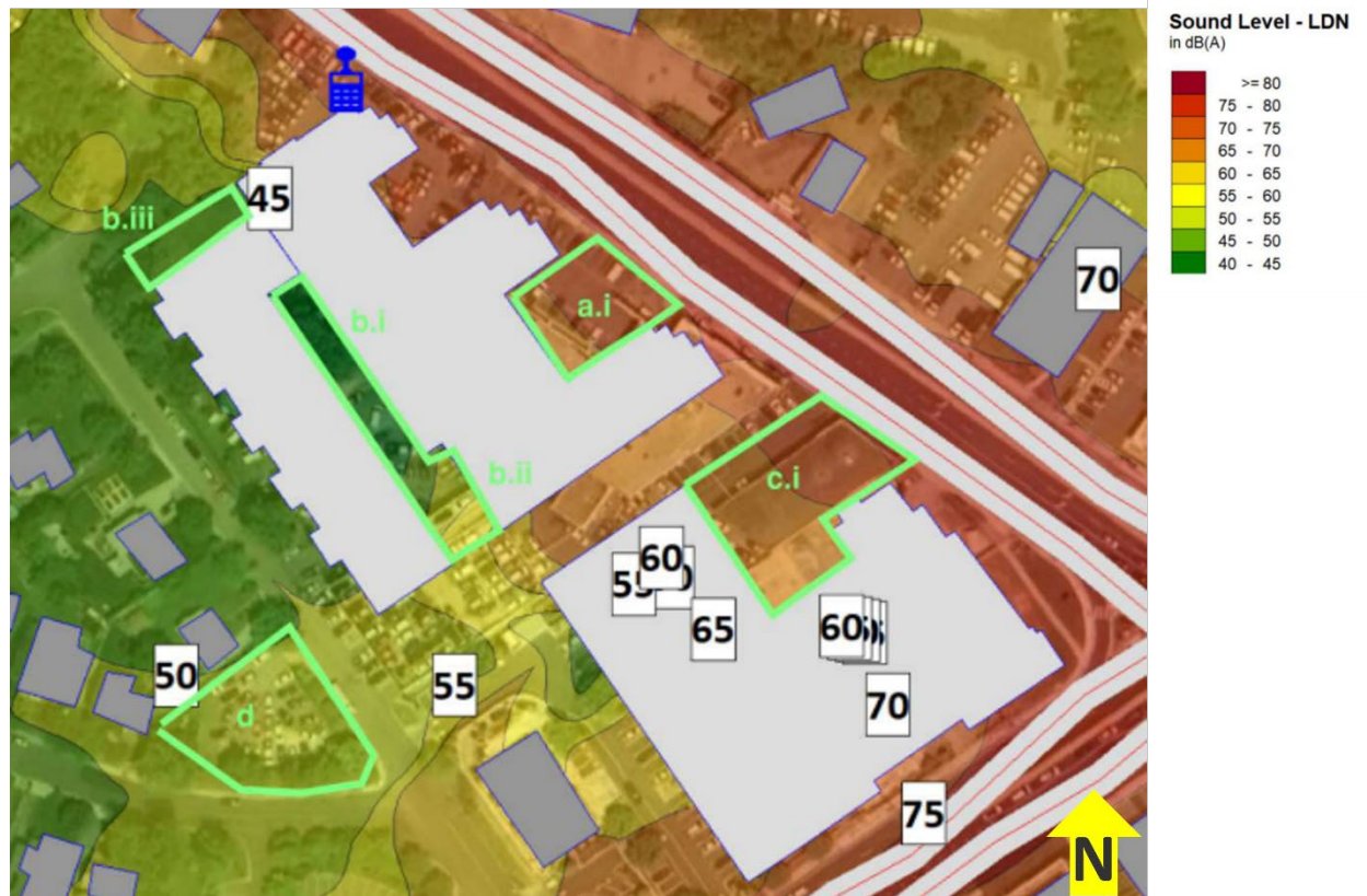
Figure 17: Projected Future Noise at Ground Level
