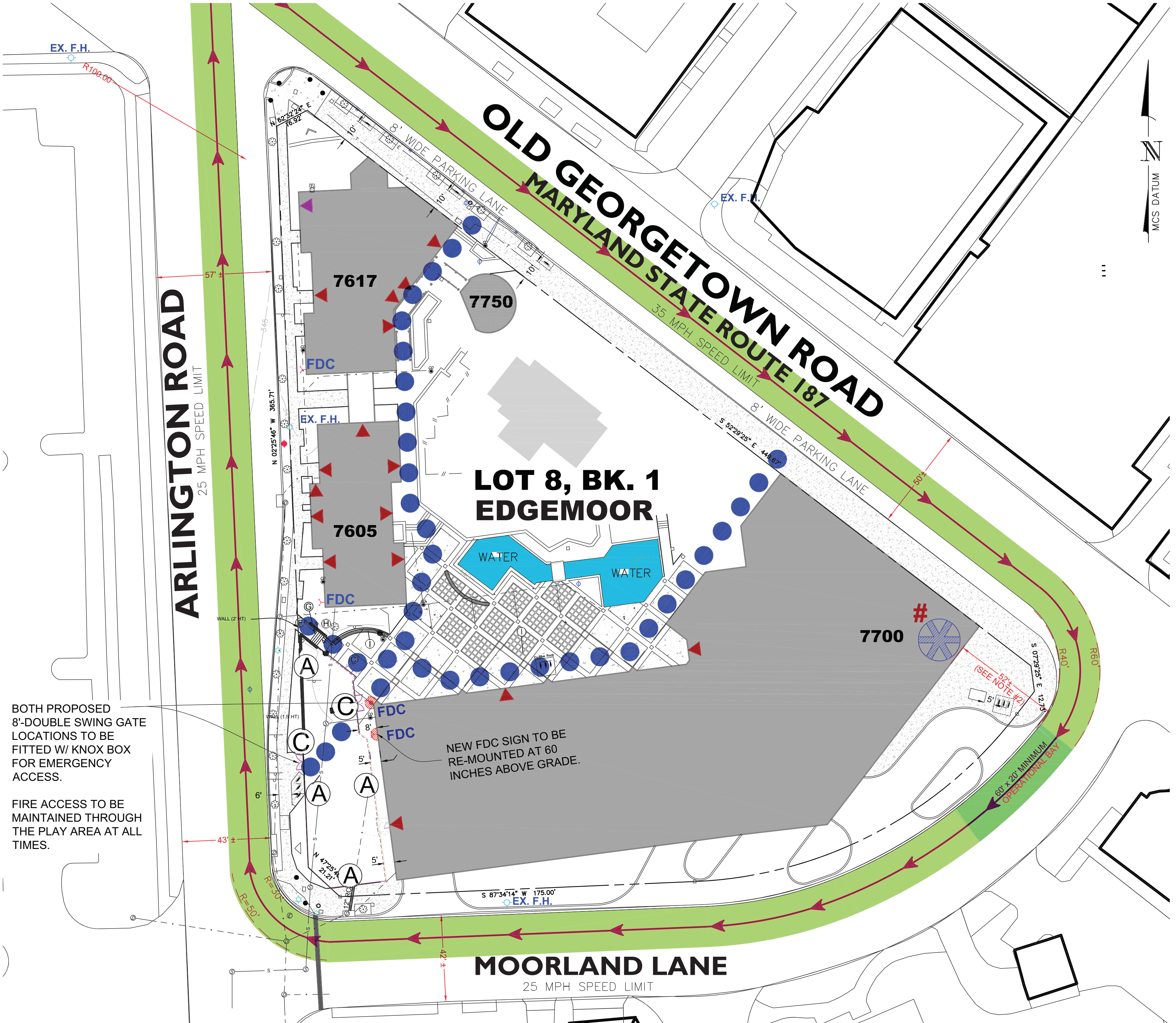
PROPOSED FIRE DEPARTMENT APPARATUS ACCESS PLAN
