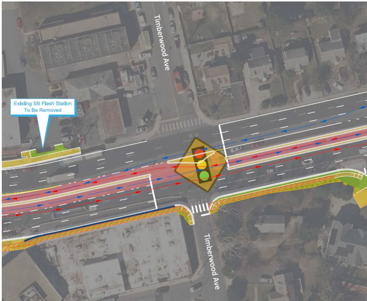
Figure 5: Transition from One Median Lane to Two Median Lanes at Timberwood Avenue
